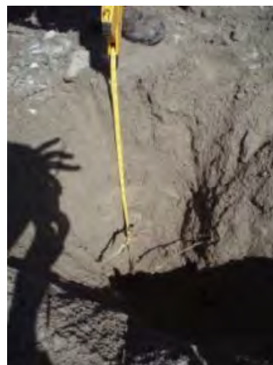
Figure 12. Soil pit in California Creek sediment plume. Lack of a visible soil horizon to depth of 26" shows lack of soil formation.
