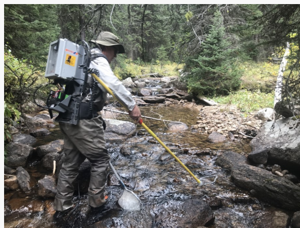
MFWP's Jim Olsen electroshocks fish in Elkhorn Creek to determine a baseline population estimate.
